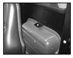
ix) Run 5/8" bulb molding provided along hood profile edge on the front panel fig.10 and along the two foot spacer box fig.11. Drop front panel on tractor fig.12. Attach Foot spacer boxes with 1/2", 1/4-20 SS Button head, and serrated flanged nut fig.13/fig.14. Leave both fasteners for bottom holes on foot spacer empty until side panels are put on. 3/4", 1/4-20 SS Button head are provided for the bottom holes.
