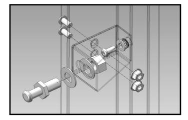
xiii) Door comes with some hardware installed fig 21. Use 2", 1/4-20 bolt, 2 washers and 1/4-20 lock nut on each door damper bracket to hold strap and buckle fig.22. Lock pin are supplied for the side panel damper bracket for quick removal of the doors fig.23.
