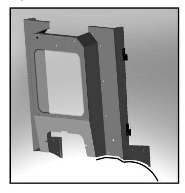
viii) With help, gently drop back assembly in place as seen in fig.8. The back panel will sit On the outside lip of the fuel tank fig.9, and fastened with the 2 bolts that were removed On both sides of the fuel tank and the one on the top. The adjustment stoppers for ROPS Can also be screwed back in place.
