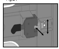
xiii) The doors can now be dropped in place and adjusted .There should be appx. 1/4" gap between door and back. 1/4" spacers can be used to hold the door in position before tightening screws. Back hinge moves up and down and door hinge moves front to back. Latch bolt bracket can be adjusted up or down fig.24 once the door is in position. Latch bolt will need to be adjusted in and out fig.24 so door closes properly with a tight seal. Door might need to be adjusted again to get a proper fit.
