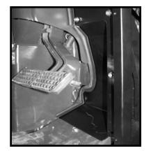
**x)** Installing the two side panels will take two people and a bit of finesse. The back and front edges of side panels need to be tucked behind the back panel fig.16 *cross section* and then the front panel fig.17 *cross section*. Install all fasteners see fig.6.
