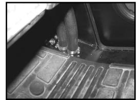
v) Use provided clips to secure heater hose along inside the cab fig.5/fig.6. Run a piece of trim along latch bolt bracket to stop hose from getting damaged fig.5.
