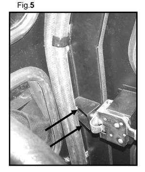
**vi)** Install 1/2" heater hose under floorboard and run to water pump fitting. Remove bypass hose from water pump and install hose fig.7.
