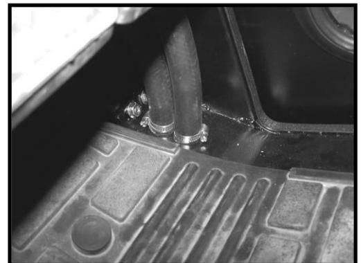
v) Use provided clips to secure heater hose along inside the cab fig.5/fig.6. Run a piece of trim along latch bolt bracket to stop hose from getting damaged fig.5.
